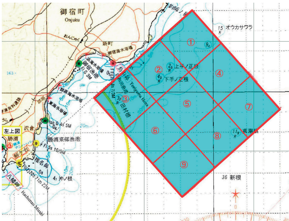
Fig. 3 Proposed survey area. The survey area by the multi-beam sonar was divided into 9 blocks, and the blocks 1, 2 and 3 were targets of the diving survey.
