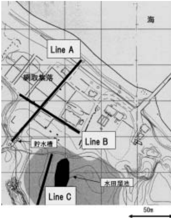
Fig. 3 The profiles( Line A, Line B, and Line C) for the dense electrical resistivity surveys.
