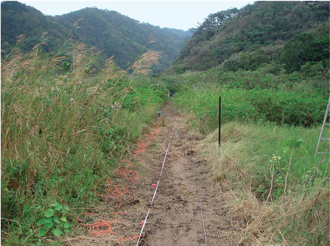
Photo 1 Along-distance view of Line A profile with geophone array in paddy fields, Amitori village.
